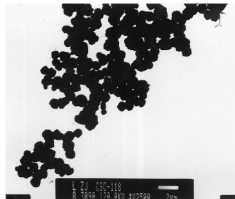
FIG. 2. TEM of micrometer-sized copper powder.
