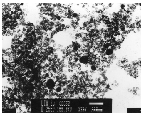
FIG. 1. TEM of nanometer-sized copper powder.
